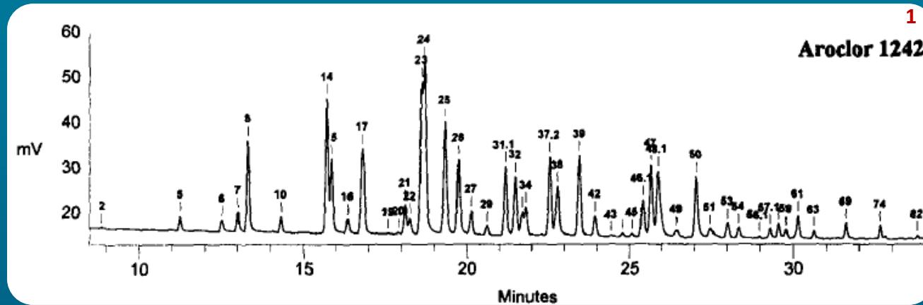
Chromatogram analyzed by a HP 5890 GC with DB-1 GC column
