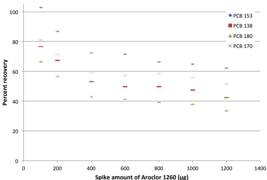
**Figure 10.** Effects of spike amount on the percent recoveries of selected PCBs in EPA 8082A mix in the absence of soil. The PCBs are extracted using headspace SPME and analyzed on the bench-top Polaris Q GC-MS (N=1).
