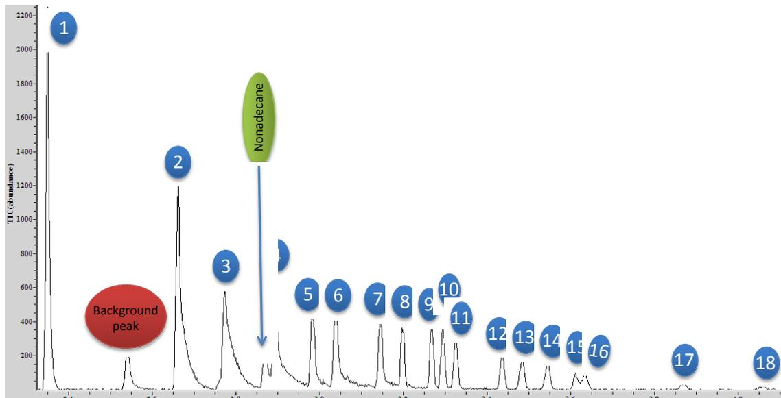
**Figure 3.** Example of headspace-SPME TIC of EPA 8082A standard (contains 19 PCB congeners) collected on the Torion Guardion<sup>®</sup>-8 GC-TMS, with nonadecane internal standard.
