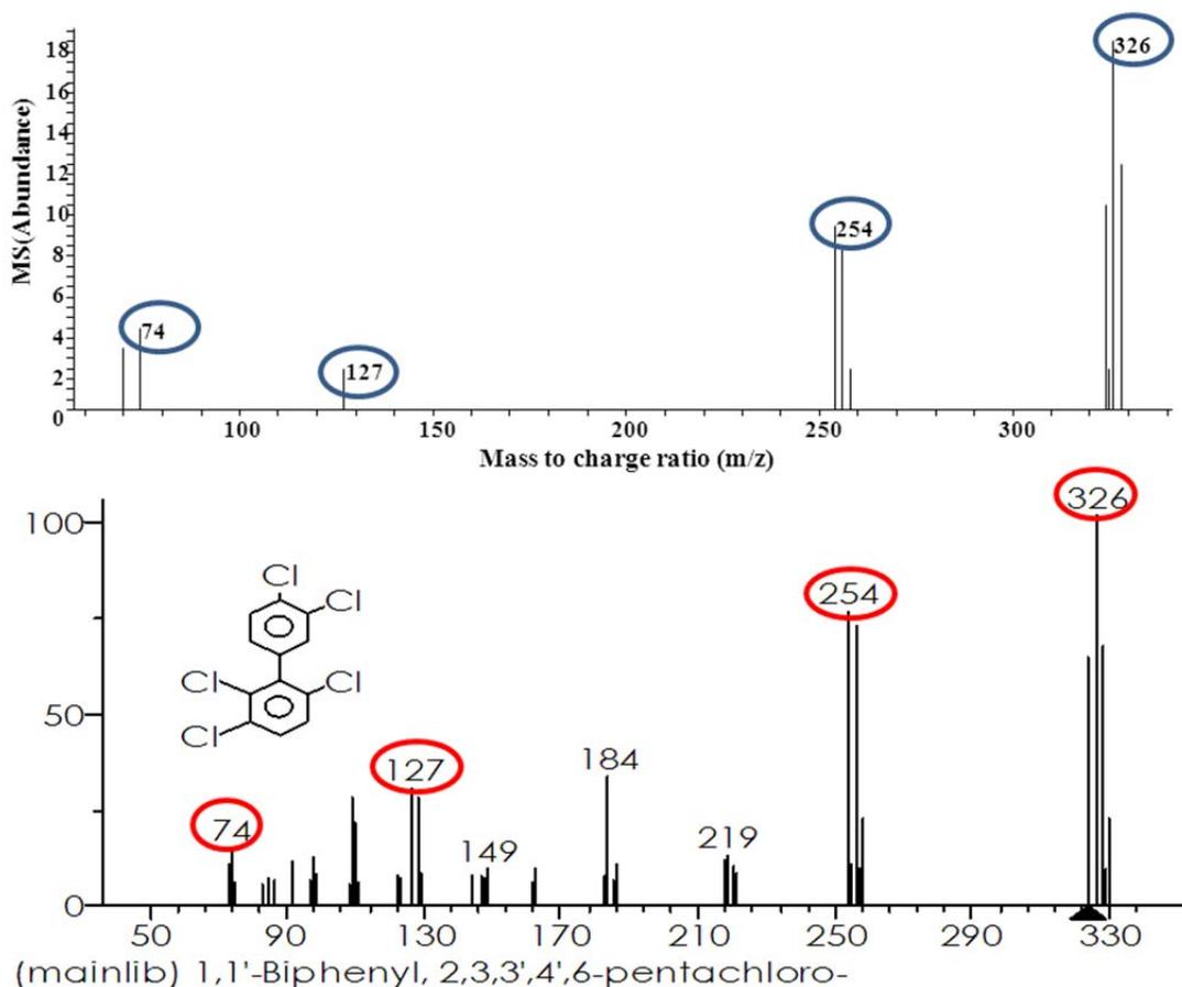
**Figure 5.** Example of mass spectra comparison for pentachlorobiphenyl between Torion Guardian®-8 GC-TMS data (top) with NIST database (bottom).
