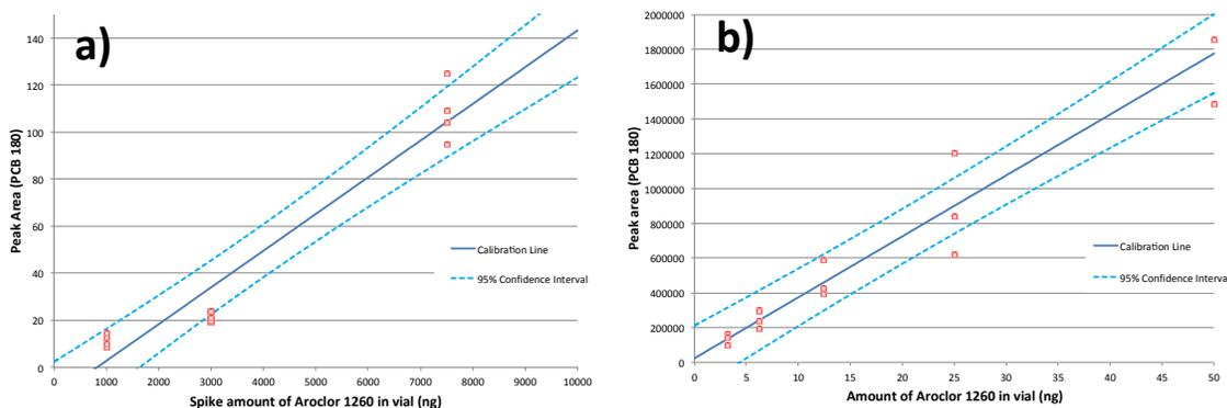
**Figure 7.** Comparisons of headspace SPME calibration curves of Aroclor 1260 for the peak tentatively assigned as PCB 180 collected on a) Portable Torion Guardian<sup>®</sup>-8 GC-TMS ( $R^2 = 0.93$ ) and b) Bench-top Thermo Polaris Q GC-MS ( $R^2 = 0.94$ ). Note that the bench-top calibration curve covers significantly lower quantities.
