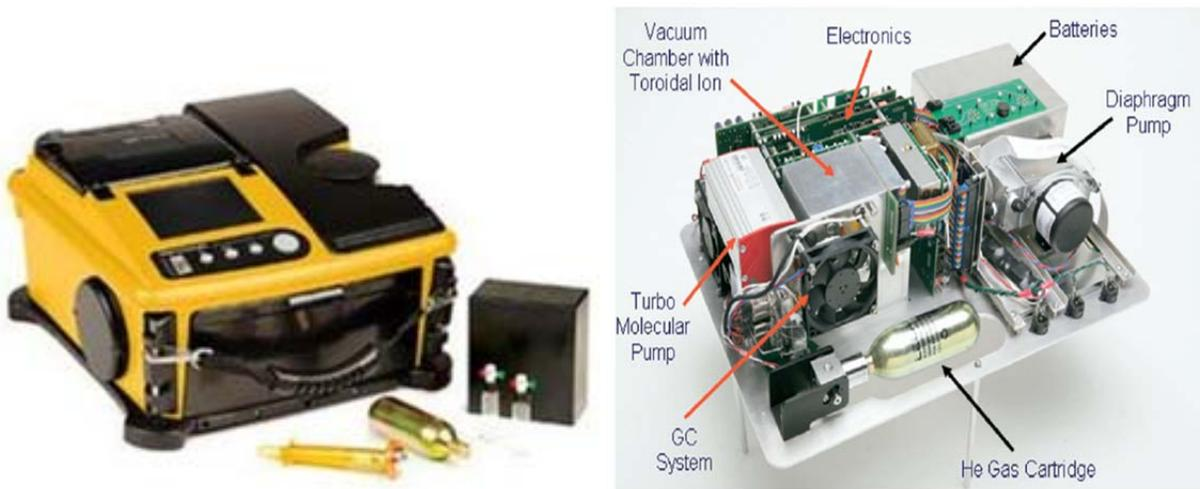
**Figure 1.** Photographs of the Guardion®-8 GC-TMS showing A) external and B) internal components.
