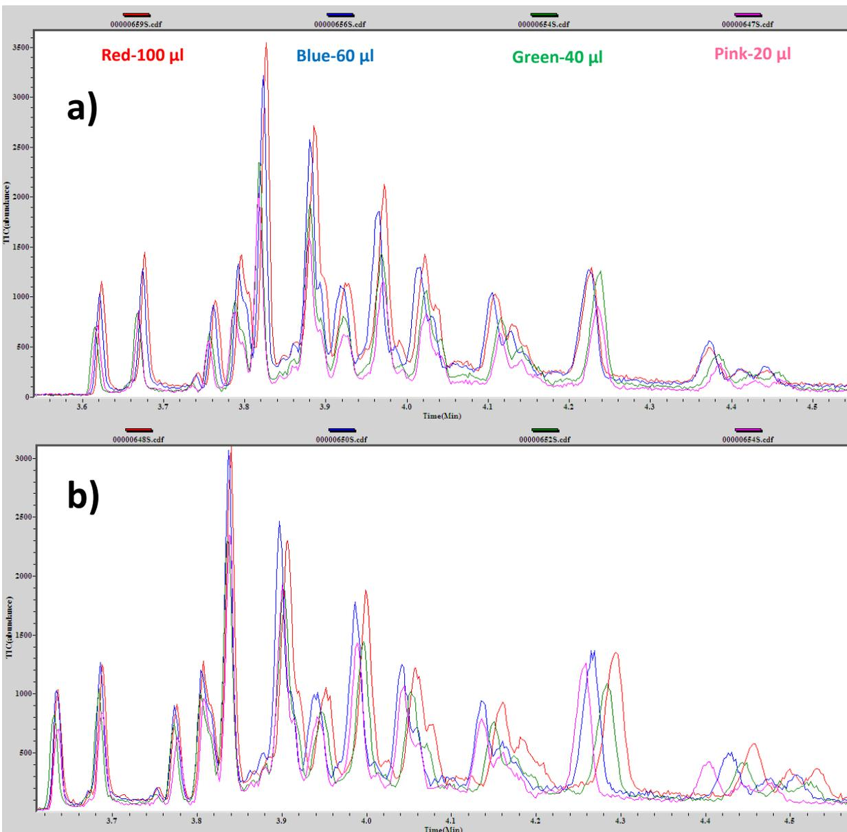
**Figure 6.** a) TIC of headspace SPME of different spike volumes of 100 ppm Aroclor 1260 standard solutions into an empty glass vial, b) Comparison of four replicate samples each at 40  $\mu$ L spike level (4  $\mu$ g Aroclor).
