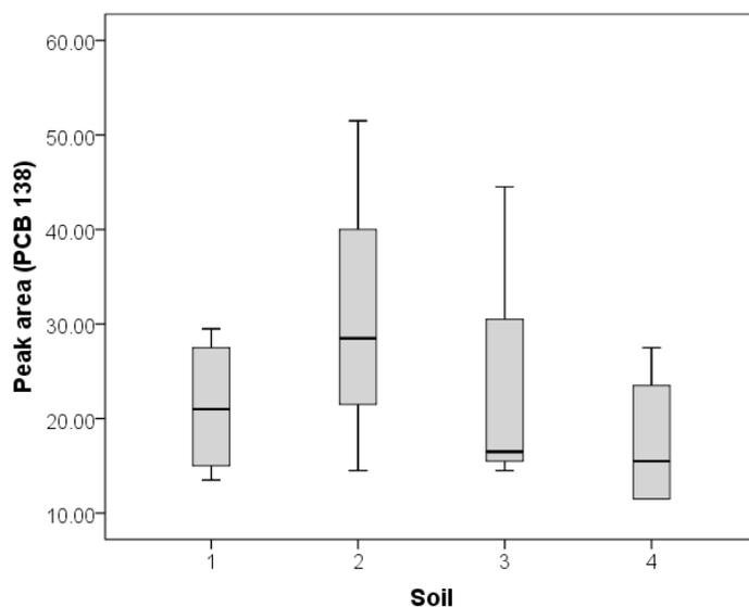
**Figure 8.** Box and whisker plot of the peak areas obtained for PCB 138 when soils for headspace SPME are prepared in different ways. Analyses performed on the Portable Torion Guardion® GC-TMS instrument.
