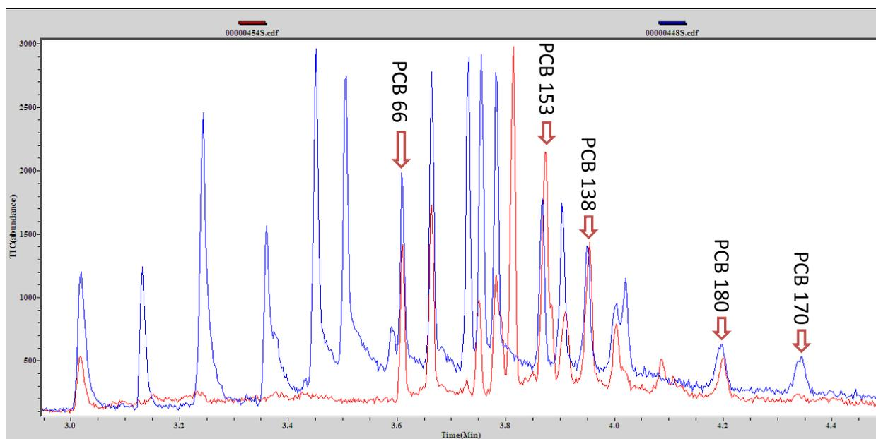
**Figure 4.** a) TIC of headspace SPME of 40  $\mu$ L of 100 ppm Aroclor 1260 (red) and EPA 8082A mix (blue) on the Torion Guardion<sup>®</sup>-8 GC-TMS. Peak assignments for the Aroclor mix (red) cannot exclude the possibility of congener co-elution.
