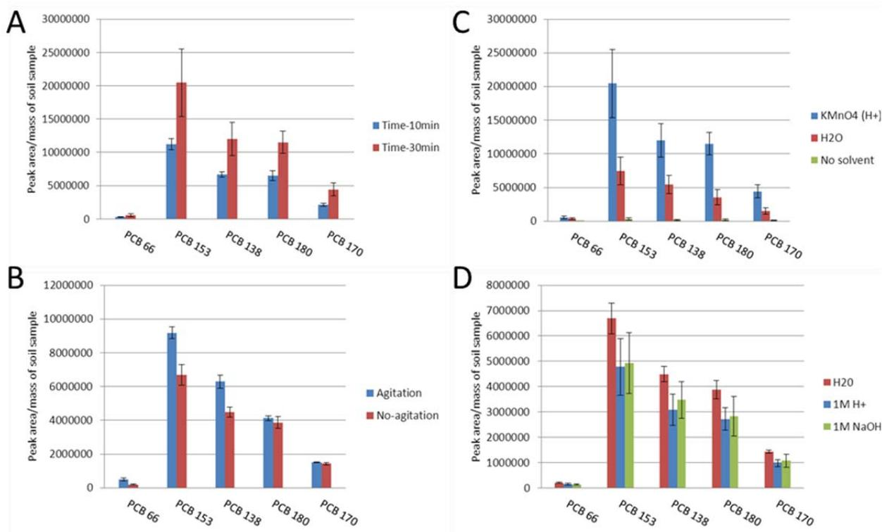
**Figure 9.** Effects of (A) SPME sorption time, (B) agitation, (C) addition of  $\text{KMnO}_4$  and  $\text{H}_2\text{O}$  and (D) addition of acid and base on extraction efficiency of PCB 66, PCB 153, PCB 138, PCB 180 and PCB 170. Error bars show  $\pm 1$  s.d. Significance tests are shown in **Table 5**.
