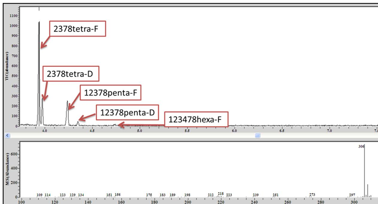
**Figure 12.** Dioxin mix standards tested on portable Torion Guardian® 8 GC-TMS system using headspace SPME extraction. Spike consisted of 50  $\mu$ L of a 5 ppm stock solution of EPA 8280B mix in the absence of soil matrix.
