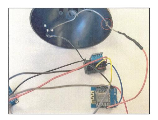
8. The lamp has an opening on its base for the OLED Display to be fitted on the outside. Place the pins for the display through the hole and rewire its pins.
