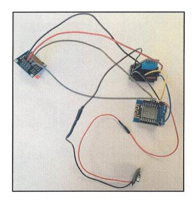
7. Wire the Lamp's positive wire (the one with the knot in it) to the D5 pin on the microcontroller.
