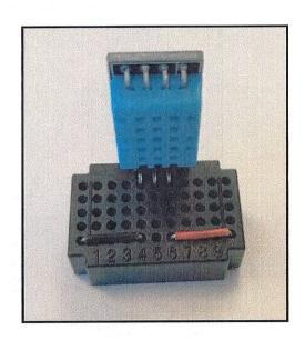
2. Use a wire to connect column 5, which is where the temperature sensor's data pin is, to the microcontroller's D3 pin.
