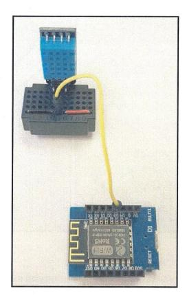
3. Connect the 3.3V power output pin on the microcontroller to the rightmost column on the breadboard.
