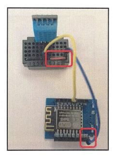
4. Connect the microcontroller's ground pin to the leftmost column of the breadboard.
